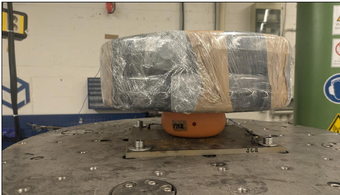
Fig 4: Exemplarily test setup for 'vibration'; PM2
