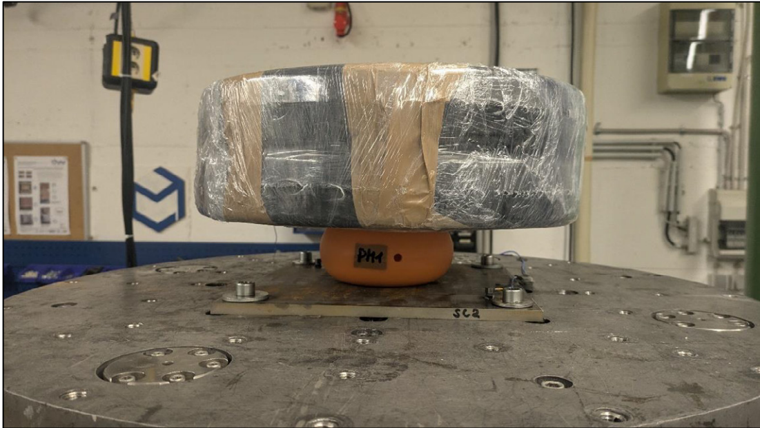
Fig 3: Exemplarily test setup for 'vibration'; PM1
