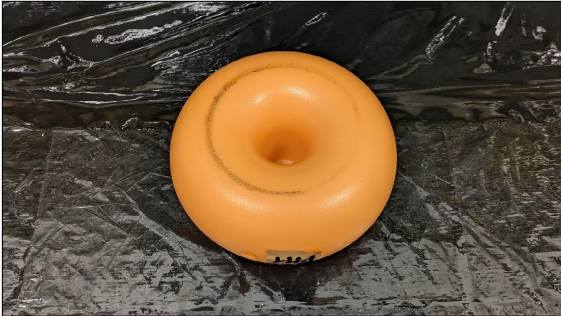
Fig 16: Visual check on completion of testing, test sample PM1, bottom view
